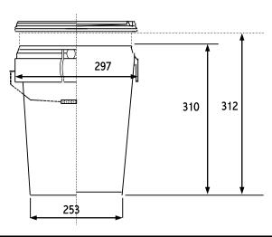
Measurements in millimetres
